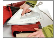
Now the patch can be sealed onto the fabric. Use an iron without steam and preheat to the highest temperature. (ca  $180^{\circ}\text{C} - 200^{\circ}\text{C}$ )
