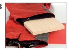
Insert a smooth and thin piece of wood. Otherwise you'll loose the pressure of the iron to the chainsaw protection.
